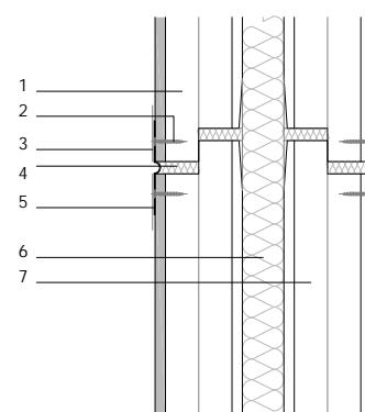
Juntas de fachada entre paneles sandwich Wallpanel CPY + lana mineral 40mm + Wallpanel YPY.
